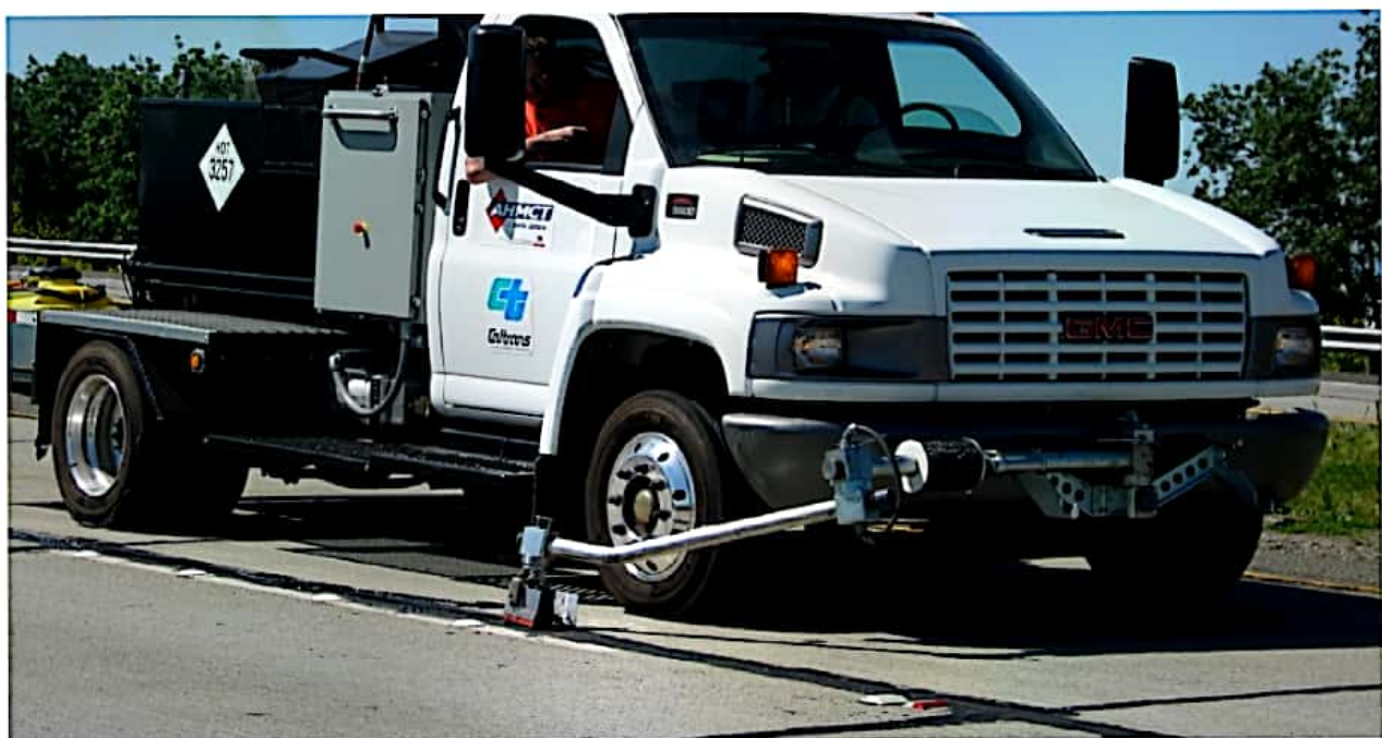
Sealzall Machine - Automated High Production Longitudinal and Manual In-Lane Crack Sealing
